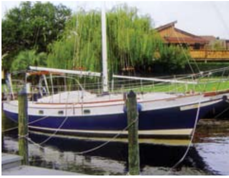
This sailboat was tied off in a canal in Gulf Breeze, Florida using three large anchors and 13 lines to shore. Despite considerable damage to other nearby boats and homes, the sailboat survived Hurricane Ivan without so much as a scratch.
